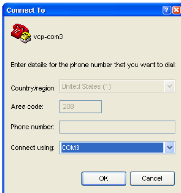
Figure 4-41 Create HyperTerminal for the virtual com port
